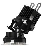
The NanoLED NXT from **USAI Lighting** provides the first 2.5-in. LED fixture with a 10 deg optic and 8,725 center beam candle power. The fixture has four beam options in 10, 25, 35 and 50 deg and has three color temperature options of 2,700, 3,000, and 3,500K.
