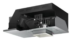
From **USAI** comes the BeveLED 2.0 Family. This complete family offers recessed downlight, adjustable and wall-wash options in three different light outputs up to 2,100 lumens. The fixture is available in four color temperatures up to 90 CRI and beam distributions of 30, 50, 80 deg.
