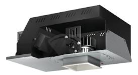
**USAI** introduces: Warm Glow Dimming in their LED downlight luminaires. A proprietary LED module shifts color temperature as the luminaire is dimmed to match the color shift of an incandescent lamp from 2,700 to 2,200K. The light engine delivers up to 63 lumens per watt in either 82 or 90 plus CRI.
