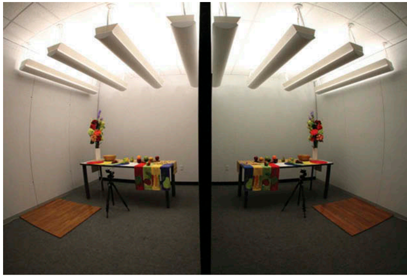
Fig. 3 Photograph taken by fish-eye lens of the full-size side-by-side rooms, viewed from the participant's standing location when performing brightness matching. A black felt curtain was behind the participant. The mirrors were hung on the dividing wall, with one in each room, which cannot be seen by the participant when performing brightness matching.
