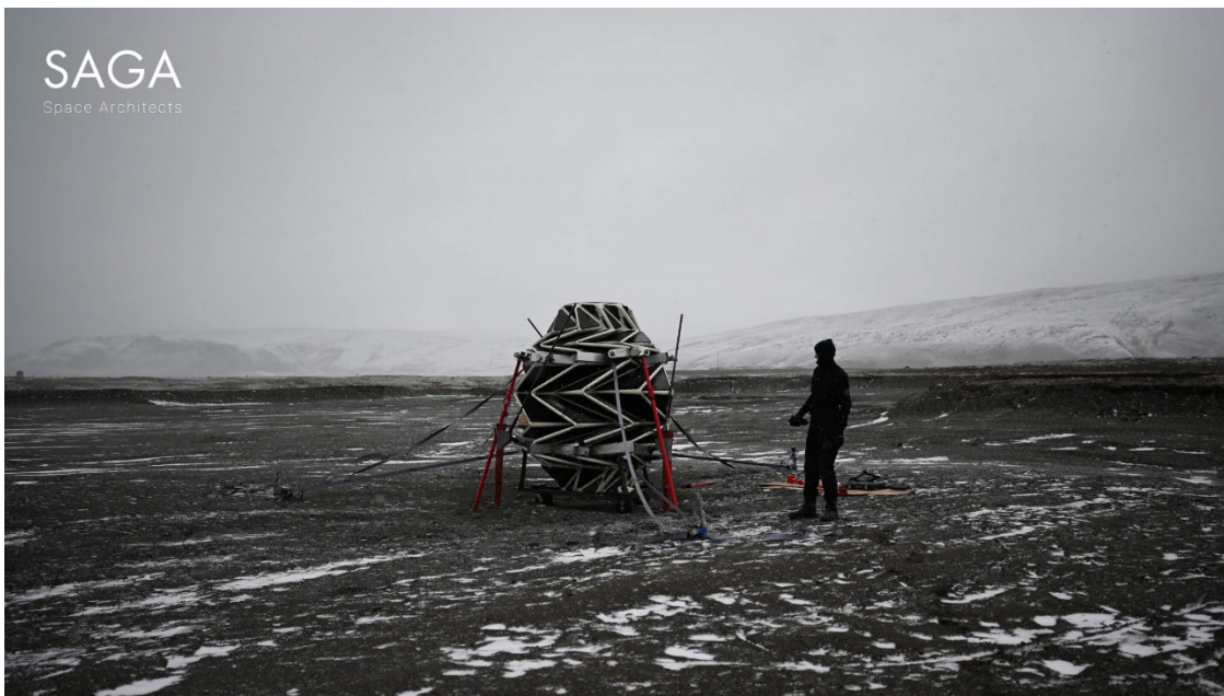
The LUNARK habitat when fully folded down and compressed (Courtesy SAGA Space Architects)
