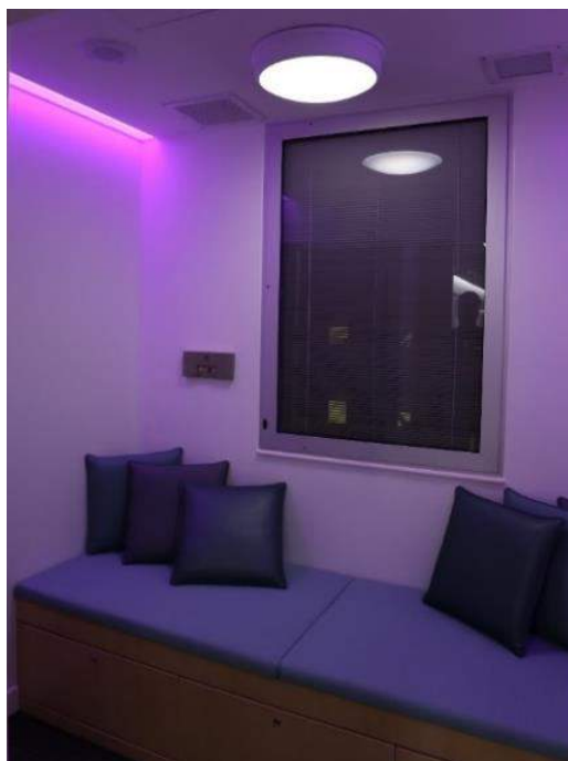
Figure 4. Serenity room. This small room provides a space for patients to spend time in a quiet space. The patients could adjust the SPD of the wall-wash luminaire to suit their mood.
