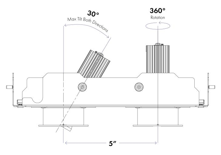
With the LittleOnes Micro Doubles Adjustable fixture, each of the two fixture heads are independently adjustable, and can be rotated 360° and tilted up to 30° maximum in either direction without interference from the other head - making lighting corners and highlighting special objects a breeze.
