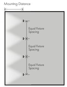
Wall Wash Mounting Recommendation: Mounting Distance = 2'-0" - 3'-6"Fixture Spacing = 2'-6" - 4'-0"
