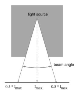
The luminous intensities are measured in a plane normal to the nominal beam centerline. If the beam is not rotationally symmetric, then the beam angle is usually given in two planes at 90° of each other, possibly the maximum and minimum angles. Other angles (eg. at 45°) may also be given.
